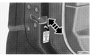
To use the system, open each rear door and slide the control UP to engage the locks and DOWN to disengage the child-protection locks. When the system on a door is engaged, that door can only be opened by using the outside door handle even if the inside door lock is in the unlocked position.
